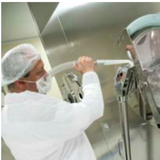
Cleaning of a coating pan.
